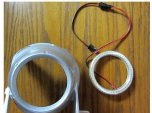
The LEDs & shroud. Cut down to the indents on the shroud to leave tabs.
