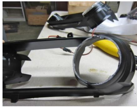
The moment of no-return. Cut the inner shroud off so the LEDs can be glued on. Leave the "tabs" for extra support for the LEDs.
